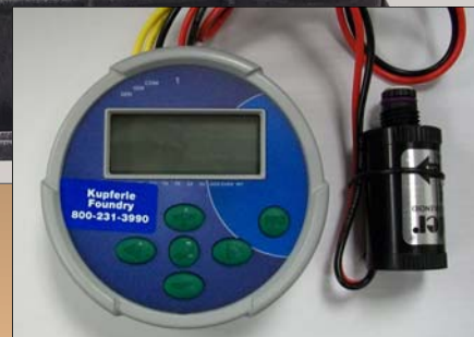
Digital Controller Allows up to 12 Flushing Cycles per day, up to 6 hours per cycle. Operates on two 9-volt batteries
